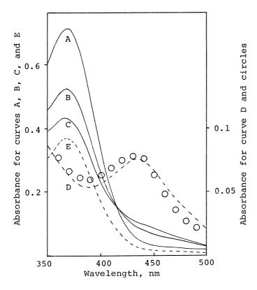
Fig. 1. Photolysis of PhSCo(dmg) $_2$ Py (47.5  $\mu$ M) in benzene solution containing pyridine (0.1 M) under anaerobic condition. A, 0 min; B, 5 min; C, 10 min. D was derived by subtracting E, corresponding to the spectrum of remaining PhSCo(dmg) $_2$ Py (24.2  $\mu$ M), from C. Circles indicate the absorbances of Co(dmg) $_2$ Py (23.3  $\mu$ M) in the same solvent. A slide projector equipped with a 650 W halogen lamp and a glass filter ( $\lambda$  > 425 nm) was used for the irradiation.
